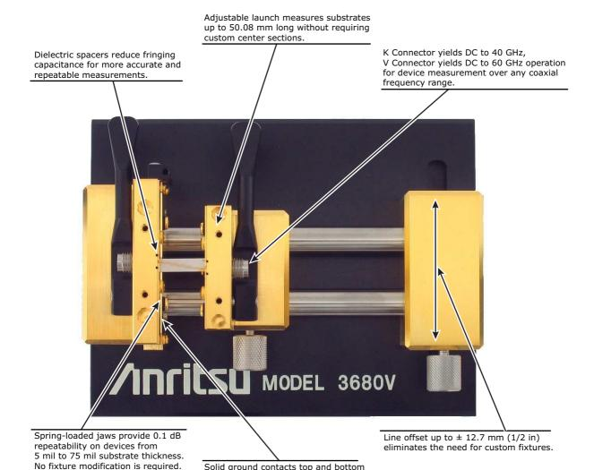
Solid ground contacts top and bottom allow microstrip or coplanar waveguide measurements in one fixture.
